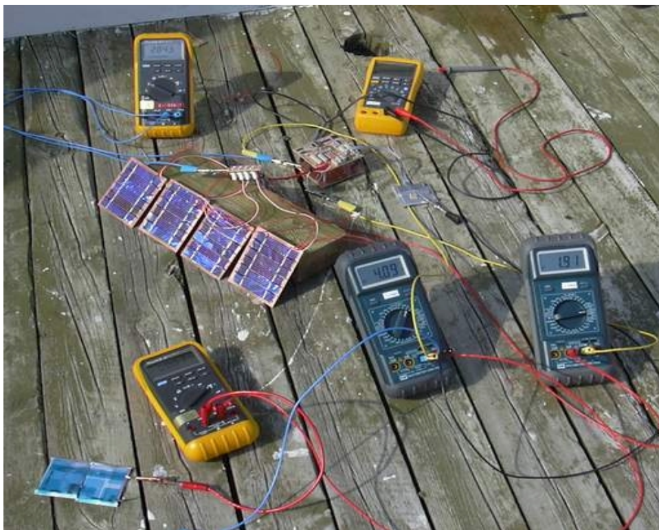
Figure 124: Here you can see the Power PCB/ backplane when the solar cells are attached and are charging the batteries.
