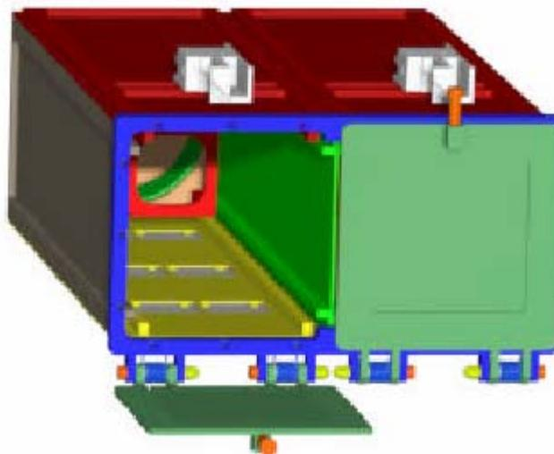
Double Barrel P-POD, Capacity of 6
