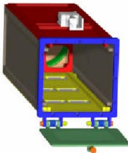
Single Barrel P-POD, Capacity of 3
