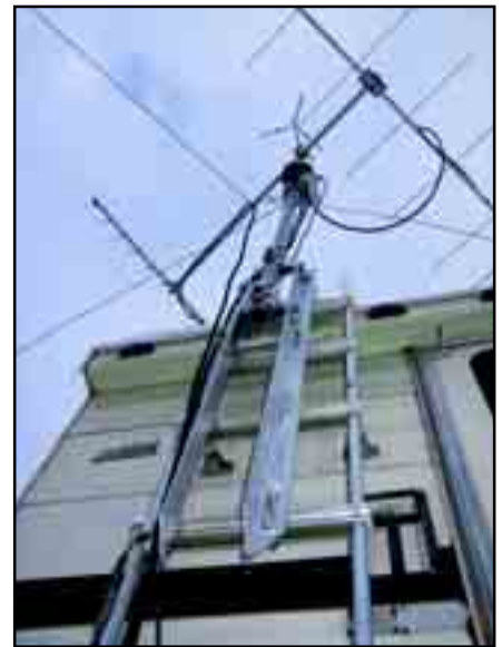
Figure 1—Gap's "Quick Tilt" ground mount was a better bet for the 60-pound antenna and rotator array since its longer legs enabled me to spread the load over four steps of my camper's ladder.
